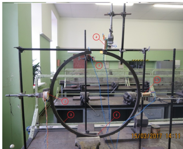
Fig. 6. Experimental board for obtaining the characteristics of the piston ring: numbering of the elements meets that of Fig. 3 of its declination
